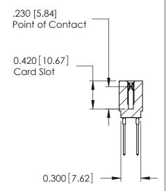
ACAD REFERENCE NO. 725-ENG MASTER 725 Series Ultra-Mate Card Edge Connector - Press Fit SEGAHOM:3A:9A DRAWN: J.LEE Part Number: 725-014-545-201 CHECKED: DATE: **EDAC INC** SCALE: SHEET 1 OF 1 THESE DRAWINGS AND SPECIFICATIONS ARE THE PROPERTY OF EDAC INC.,AND TORONTO, ONTARIO SHALL NOT BE REPRODUCED, OR COPIED DRAWING NUMBER **ISSUE** CANADA OR USED AS THE BASIS FOR THE 725-ENG MASTER MANUFACTURE OR SALE OF APPARATUS YOUR CONNECTION TO QUALITY & SERVICE WITHOUT WRITTEN PERMISSION.
