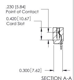
725 Series Ultra-Mate Card Edge Connector - Press Fit
