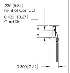
725 Series Ultra-Mate Card Edge Connector - Press Fit Part Number: 725-015-541-101
