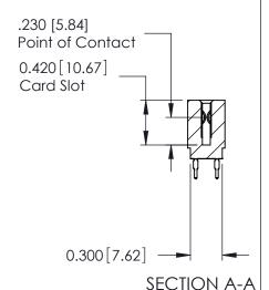
725 Series Ultra-Mate Card Edge Connector - Press Fit ACAD REFERENCE NO.
