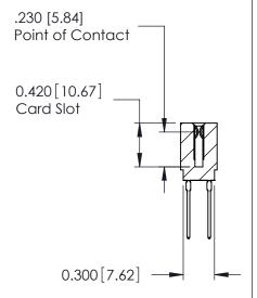
ACAD REFERENCE NO. 725-ENG MASTER 725 Series Ultra-Mate Card Edge Connector - Press Fit SEGAHOM:3A:9A DRAWN: J.LEE Part Number: 725-020-545-201 CHECKED: DATE: **EDAC INC** SCALE: SHEET 1 OF 1 THESE DRAWINGS AND SPECIFICATIONS ARE THE PROPERTY OF EDAC INC.,AND TORONTO, ONTARIO SHALL NOT BE REPRODUCED, OR COPIED DRAWING NUMBER **ISSUE** CANADA OR USED AS THE BASIS FOR THE 725-ENG MASTER MANUFACTURE OR SALE OF APPARATUS YOUR CONNECTION TO QUALITY & SERVICE WITHOUT WRITTEN PERMISSION.
