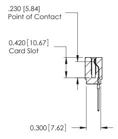
ACAD REFERENCE NO. 725-ENG MASTER 725 Series Ultra-Mate Card Edge Connector - Press Fit SEGAHON:3A:9A DRAWN: J.LEE Part Number: 725-022-545-101 CHECKED: DATE: SCALE: **EDAC INC** SHEET 1 OF 1 THESE DRAWINGS AND SPECIFICATIONS ARE THE PROPERTY OF EDAC INC., AND TORONTO, ONTARIO SHALL NOT BE REPRODUCED, OR COPIED DRAWING NUMBER **ISSUE** CANADA OR USED AS THE BASIS FOR THE 725-ENG MASTER MANUFACTURE OR SALE OF APPARATUS YOUR CONNECTION TO QUALITY & SERVICE WITHOUT WRITTEN PERMISSION.
