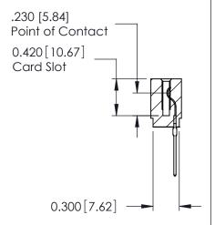
ACAD REFERENCE NO. 725 Series Ultra-Mate Card Edge Connector - Press Fit Part Number: 725-023-540-101 **EDAC INC** THESE DRAWINGS AND SPECIFICATIONS
