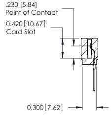
ACAD REFERENCE NO. 725-ENG MASTER 725 Series Ultra-Mate Card Edge Connector - Press Fit SEGAHOM:3A:9A DRAWN: J.LEE Part Number: 725-026-540-101 CHECKED: DATE: SCALE: **EDAC INC** SHEET 1 OF 1 THESE DRAWINGS AND SPECIFICATIONS ARE THE PROPERTY OF EDAC INC.,AND TORONTO, ONTARIO SHALL NOT BE REPRODUCED, OR COPIED DRAWING NUMBER **ISSUE** CANADA OR USED AS THE BASIS FOR THE 725-ENG MASTER MANUFACTURE OR SALE OF APPARATUS YOUR CONNECTION TO QUALITY & SERVICE WITHOUT WRITTEN PERMISSION.
