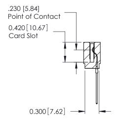
725 Series Ultra-Mate Card Edge Connector - Press Fit Part Number: 725-026-541-101 **EDAC INC** THESE DRAWINGS AND SPECIFICATIONS
