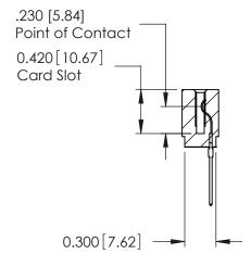
ACAD REFERENCE NO. 725-ENG MASTER 725 Series Ultra-Mate Card Edge Connector - Press Fit SEGAHOM:3A:9A DRAWN: J.LEE Part Number: 725-029-540-101 CHECKED: DATE: SCALE: **EDAC INC** SHEET 1 OF 1 THESE DRAWINGS AND SPECIFICATIONS ARE THE PROPERTY OF EDAC INC.,AND TORONTO, ONTARIO SHALL NOT BE REPRODUCED, OR COPIED DRAWING NUMBER **ISSUE** CANADA OR USED AS THE BASIS FOR THE 725-ENG MASTER MANUFACTURE OR SALE OF APPARATUS YOUR CONNECTION TO QUALITY & SERVICE WITHOUT WRITTEN PERMISSION.
