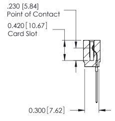
725 Series Ultra-Mate Card Edge Connector - Press Fit Part Number: 725-029-541-101
