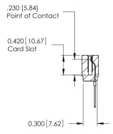
725 Series Ultra-Mate Card Edge Connector - Press Fit Part Number: 725-030-545-101
