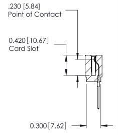
725 Series Ultra-Mate Card Edge Connector - Press Fit
