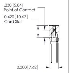
ACAD REFERENCE NO. 725 Series Ultra-Mate Card Edge Connector - Press Fit DRAWN: J.LEE Part Number: 725-040-541-201 CHECKED: **EDAC INC** THESE DRAWINGS AND SPECIFICATIONS
