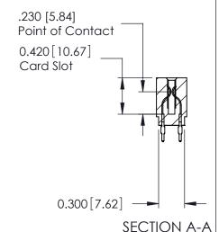
ACAD REFERENCE NO. 725 Series Ultra-Mate Card Edge Connector - Press Fit
