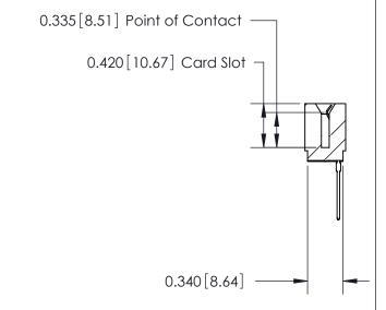
ACAD REFERENCE NO. 726 Series Ultra-Mate Card Edge Connector - Press Fit DRAWN: J.LEE Part Number: 726-011-545-101 CHECKED: **EDAC INC** SCALE: THESE DRAWINGS AND SPECIFICATIONS ARE THE PROPERTY OF EDAC INC.,AND TORONTO, ONTARIO SHALL NOT BE REPRODUCED, OR COPIED DRAWING NUMBER CANADA OR USED AS THE BASIS FOR THE 726-ENG MASTER MANUFACTURE OR SALE OF APPARATUS YOUR CONNECTION TO QUALITY & SERVICE WITHOUT WRITTEN PERMISSION.
