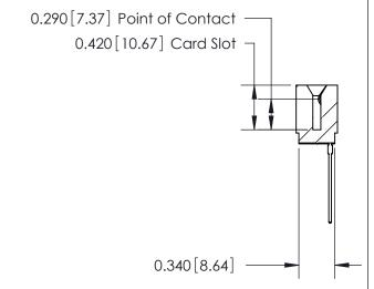
726 Series Ultra-Mate Card Edge Connector - Press Fit Part Number: 726-013-541-101 **EDAC INC** THESE DRAWINGS AND SPECIFICATIONS ARE THE PROPERTY OF EDAC INC.,AND TORONTO, ONTARIO SHALL NOT BE REPRODUCED, OR COPIED CANADA OR USED AS THE BASIS FOR THE MANUFACTURE OR SALE OF APPARATUS YOUR CONNECTION TO QUALITY & SERVICE WITHOUT WRITTEN PERMISSION.
