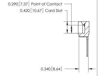
ACAD REFERENCE NO. 726 Series Ultra-Mate Card Edge Connector - Press Fit DRAWN: Part Number: 726-016-553-101 **EDAC INC** THESE DRAWINGS AND SPECIFICATIONS ARE THE PROPERTY OF EDAC INC.,AND TORONTO, ONTARIO SHALL NOT BE REPRODUCED, OR COPIED CANADA OR USED AS THE BASIS FOR THE MANUFACTURE OR SALE OF APPARATUS YOUR CONNECTION TO QUALITY & SERVICE WITHOUT WRITTEN PERMISSION.
