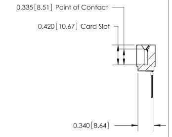
726 Series Ultra-Mate Card Edge Connector - Press Fit Part Number: 726-020-545-101 **EDAC INC** THESE DRAWINGS AND SPECIFICATIONS ARE THE PROPERTY OF EDAC INC., AND
