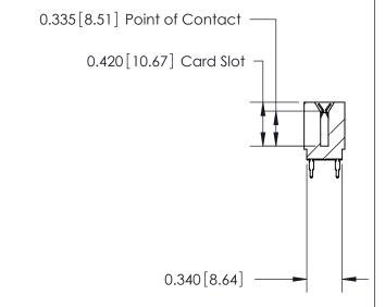
ACAD REFERENCE NO. 726 Series Ultra-Mate Card Edge Connector - Press Fit DRAWN: J.LEE Part Number: 726-022-525-201 CHECKED: **EDAC INC** SCALE: THESE DRAWINGS AND SPECIFICATIONS ARE THE PROPERTY OF EDAC INC., AND TORONTO, ONTARIO SHALL NOT BE REPRODUCED, OR COPIED DRAWING NUMBER CANADA OR USED AS THE BASIS FOR THE 726-ENG MASTER MANUFACTURE OR SALE OF APPARATUS YOUR CONNECTION TO QUALITY & SERVICE WITHOUT WRITTEN PERMISSION.
