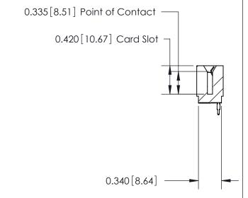
726 Series Ultra-Mate Card Edge Connector - Press Fit Part Number: 726-025-525-101
