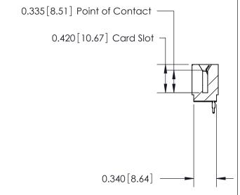
726 Series Ultra-Mate Card Edge Connector - Press Fit Part Number: 726-030-525-101 **EDAC INC** THESE DRAWINGS AND SPECIFICATIONS
