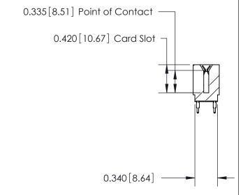
726 Series Ultra-Mate Card Edge Connector - Press Fit ACAD REFERENCE NO. 726-ENG MASTER Part Number: 726-044-525-201
