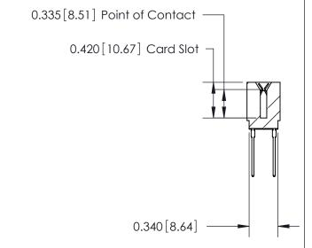
726 Series Ultra-Mate Card Edge Connector - Press Fit Part Number: 726-050-545-201 **EDAC INC** THESE DRAWINGS AND SPECIFICATIONS ARE THE PROPERTY OF EDAC INC.,AND TORONTO, ONTARIO
