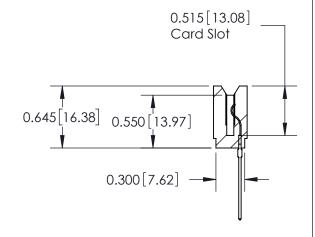
737 Series Ultra-Mate Card Edge Connector - Press Fit ACAD REFERENCE NO. 737-ENG MASTER
