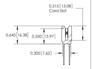
ACAD REFERENCE NO. 737 Series Ultra-Mate Card Edge Connector - Press Fit DRAWN: Part Number: 737-022-541-206 CHECKED: **EDAC INC** SCALE: THESE DRAWINGS AND SPECIFICATIONS ARE THE PROPERTY OF EDAC INC.,AND TORONTO, ONTARIO SHALL NOT BE REPRODUCED, OR COPIED DRAWING NUMBER CANADA OR USED AS THE BASIS FOR THE MANUFACTURE OR SALE OF APPARATUS YOUR CONNECTION TO QUALITY & SERVICE WITHOUT WRITTEN PERMISSION.
