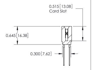
ACAD REFERENCE NO. 737 Series Ultra-Mate Card Edge Connector - Press Fit DRAWN: Part Number: 737-024-541-201 CHECKED: **EDAC INC** SCALE: THESE DRAWINGS AND SPECIFICATIONS ARE THE PROPERTY OF EDAC INC.,AND TORONTO, ONTARIO SHALL NOT BE REPRODUCED, OR COPIED DRAWING NUMBER CANADA OR USED AS THE BASIS FOR THE MANUFACTURE OR SALE OF APPARATUS YOUR CONNECTION TO QUALITY & SERVICE WITHOUT WRITTEN PERMISSION.
