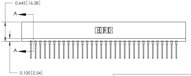
737 Series Ultra-Mate Card Edge Connector - Press Fit
