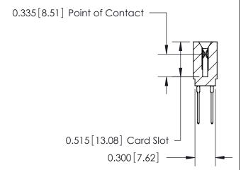
ACAD REFERENCE NO. 745 Series Ultra-Mate Card Edge Connector - Press Fit DRAWN: J.LEE Part Number: 745-010-545-201 CHECKED: **EDAC INC** SCALE: THESE DRAWINGS AND SPECIFICATIONS ARE THE PROPERTY OF EDAC INC.,AND TORONTO, ONTARIO SHALL NOT BE REPRODUCED, OR COPIED DRAWING NUMBER CANADA OR USED AS THE BASIS FOR THE 745-ENG MASTER MANUFACTURE OR SALE OF APPARATUS YOUR CONNECTION TO QUALITY & SERVICE WITHOUT WRITTEN PERMISSION.
