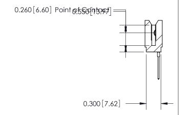
ACAD REFERENCE NO. 745 Series Ultra-Mate Card Edge Connector - Press Fit DRAWN: J.LEE Part Number: 745-012-540-106 CHECKED: **EDAC INC** SCALE: THESE DRAWINGS AND SPECIFICATIONS ARE THE PROPERTY OF EDAC INC.,AND TORONTO, ONTARIO SHALL NOT BE REPRODUCED, OR COPIED DRAWING NUMBER CANADA OR USED AS THE BASIS FOR THE 745-ENG MASTER MANUFACTURE OR SALE OF APPARATUS YOUR CONNECTION TO QUALITY & SERVICE WITHOUT WRITTEN PERMISSION.
