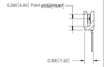
ACAD REFERENCE NO. 745 Series Ultra-Mate Card Edge Connector - Press Fit DRAWN: DATE: MAY 04/09 J.LEE Part Number: 745-012-541-106 CHECKED: DATE: **EDAC INC** SCALE: SHEET 1 OF 2 THESE DRAWINGS AND SPECIFICATIONS ARE THE PROPERTY OF EDAC INC.,AND TORONTO, ONTARIO SHALL NOT BE REPRODUCED, OR COPIED DRAWING NUMBER CANADA OR USED AS THE BASIS FOR THE 745-ENG MASTER MANUFACTURE OR SALE OF APPARATUS YOUR CONNECTION TO QUALITY & SERVICE WITHOUT WRITTEN PERMISSION.
