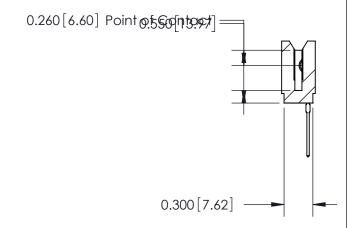
745 Series Ultra-Mate Card Edge Connector - Press Fit Part Number: 745-046-540-106
