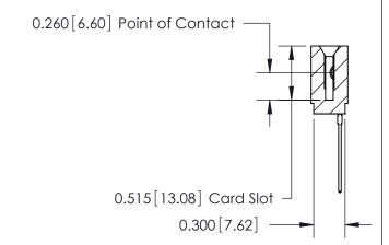
745 Series Ultra-Mate Card Edge Connector - Press Fit Part Number: 745-046-541-101
