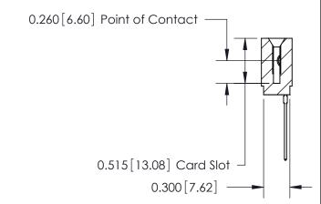
745 Series Ultra-Mate Card Edge Connector - Press Fit Part Number: 745-047-541-101
