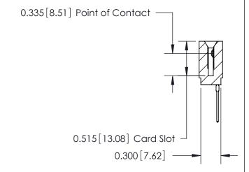
745 Series Ultra-Mate Card Edge Connector - Press Fit ACAD REFERENCE NO.
