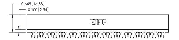
745 Series Ultra-Mate Card Edge Connector - Press Fit Part Number: 745-049-520-101 **EDAC INC** THESE DRAWINGS AND SPECIFICATIONS ARE THE PROPERTY OF EDAC INC.,AND TORONTO, ONTARIO
