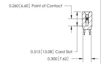
ACAD REFERENCE NO. 745 Series Ultra-Mate Card Edge Connector - Press Fit DRAWN: J.LEE Part Number: 745-082-520-201 CHECKED: SCALE: **EDAC INC** THESE DRAWINGS AND SPECIFICATIONS ARE THE PROPERTY OF EDAC INC.,AND TORONTO, ONTARIO SHALL NOT BE REPRODUCED, OR COPIED DRAWING NUMBER CANADA OR USED AS THE BASIS FOR THE 745-ENG MASTER MANUFACTURE OR SALE OF APPARATUS YOUR CONNECTION TO QUALITY & SERVICE WITHOUT WRITTEN PERMISSION.
