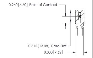
745 Series Ultra-Mate Card Edge Connector - Press Fit
