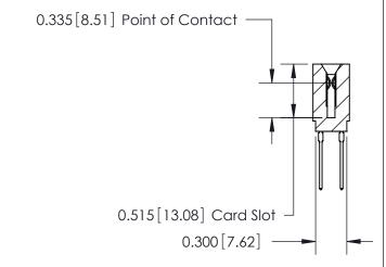
745 Series Ultra-Mate Card Edge Connector - Press Fit ACAD REFERENCE NO. Part Number: 745-088-545-201
