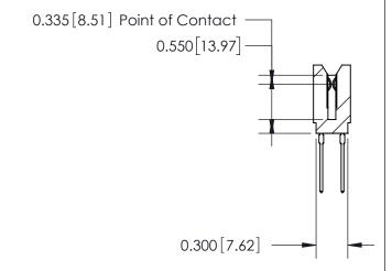
745 Series Ultra-Mate Card Edge Connector - Press Fit ACAD REFERENCE NO. Part Number: 745-088-545-206 **EDAC INC** THESE DRAWINGS AND SPECIFICATIONS
