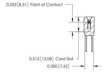
745 Series Ultra-Mate Card Edge Connector - Press Fit Part Number: 745-098-545-201
