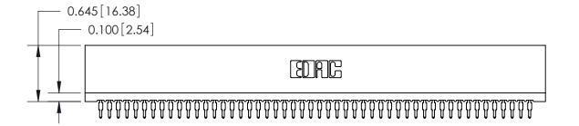
745 Series Ultra-Mate Card Edge Connector - Press Fit Part Number: 745-100-520-201
