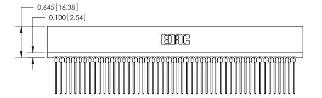
745 Series Ultra-Mate Card Edge Connector - Press Fit
