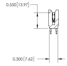
745 Series Ultra-Mate Card Edge Connector - Press Fit Part Number: 745-100-560-206 **EDAC INC** THESE DRAWINGS AND SPECIFICATIONS
