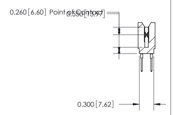
745 Series Ultra-Mate Card Edge Connector - Press Fit Part Number: 745-102-522-206 **EDAC INC** THESE DRAWINGS AND SPECIFICATIONS
