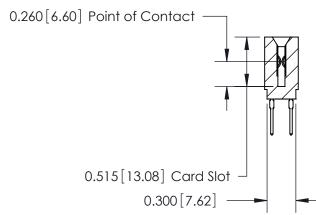
745 Series Ultra-Mate Card Edge Connector - Press Fit Part Number: 745-104-522-201 THESE DRAWINGS AND SPECIFICATIONS
