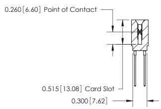
745 Series Ultra-Mate Card Edge Connector - Press Fit
