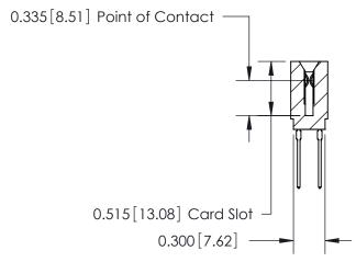
745 Series Ultra-Mate Card Edge Connector - Press Fit
