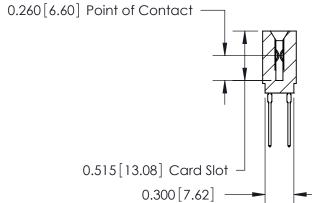
745 Series Ultra-Mate Card Edge Connector - Press Fit Part Number: 745-106-540-201
