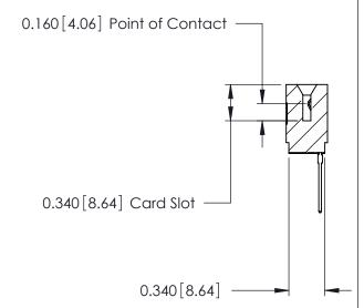
ACAD REFERENCE NO. 746-ENG MASTER 746 Series Ultra-Mate Card Edge Connector - Press Fit DRAWN: DATE: AUG 20/09 J.LEE Part Number: 746-005-545-501 CHECKED: DATE: **EDAC INC** SCALE: SHEET 1 OF 1 THESE DRAWINGS AND SPECIFICATIONS ARE THE PROPERTY OF EDAC INC.,AND TORONTO, ONTARIO SHALL NOT BE REPRODUCED, OR COPIED DRAWING NUMBER **ISSUE** CANADA OR USED AS THE BASIS FOR THE 746-ENG MASTER MANUFACTURE OR SALE OF APPARATUS YOUR CONNECTION TO QUALITY & SERVICE WITHOUT WRITTEN PERMISSION.
